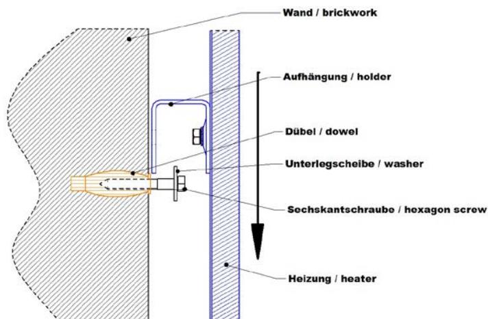
**II. Turn the outer holders on the bottom side for 90°. This will fix the heater to the wall (see sketch above).**
