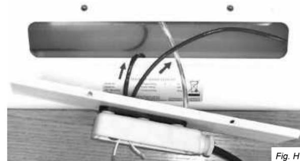
5. Pull the emitter wires one at a time through the plate to remove as shown in Fig. H.
