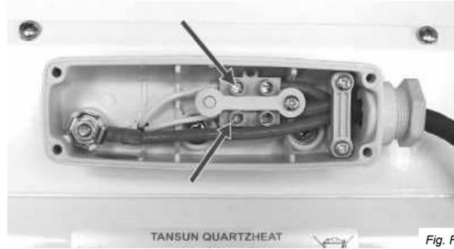
3. Disconnect the emitter from the connector blocks by unscrewing the screws highlighted above in Fig. F and remove the white coloured emitter wires from the terminal block.
